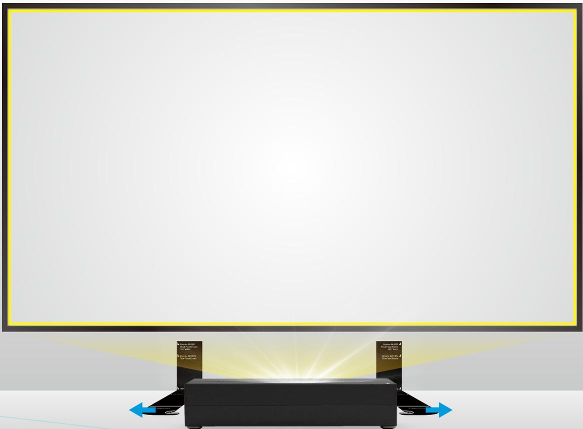
8. Mount the Fixed Frame Screen to the Wall using the yellow screen pattern as a guide.
