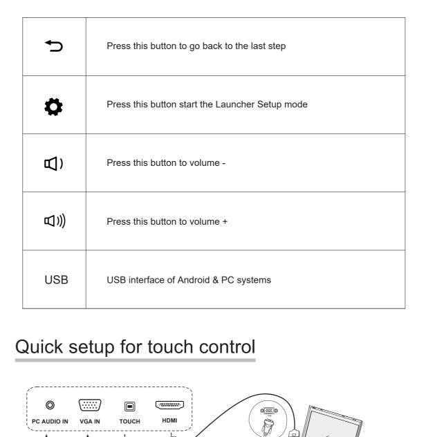
Use a VGA or HDMI cable, USB cable, and Audio cable to connect between an external computer and
